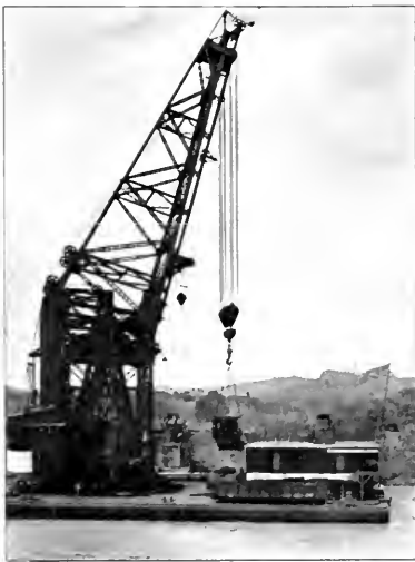
One of the Canal Commission's big floating cranes handling railroad equipment.
